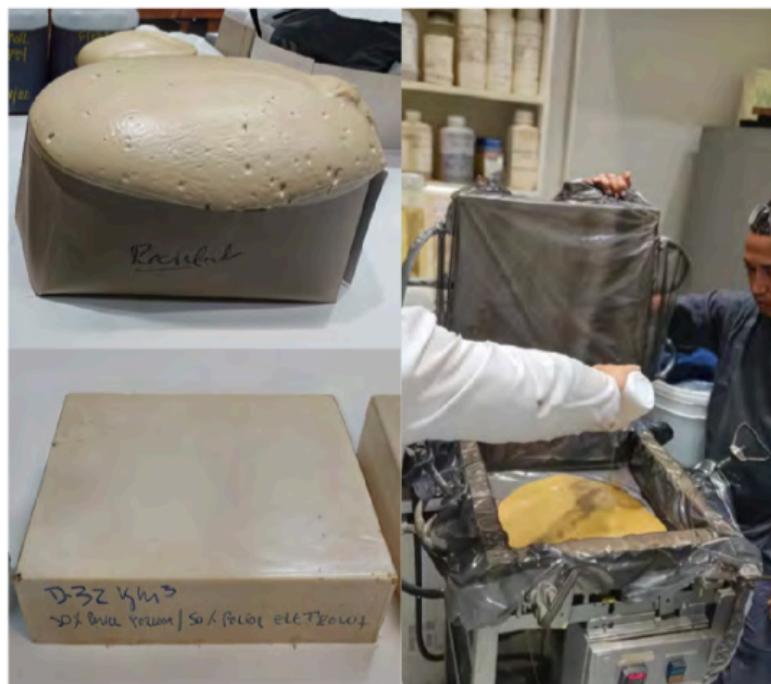
Figure 5: Laboratory production of foam test blocks
